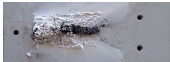
Figure 6.2: the same coating but with a different sample preparation procedure. Sample failed the same stress as the one applied in 6.1
