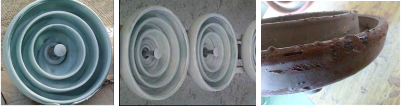
Figure 9: Examples of visual defects in the application. (left: uncoated areas, center: uneven coating, right: runners and droplets)
