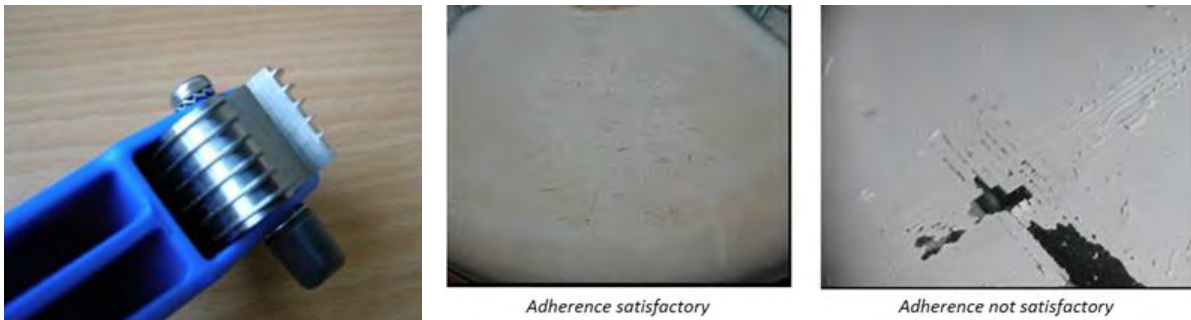
Figure 11: Scratch test as per ISO-EN2409. Left: testing fork. Center: acceptable adherence. Right: Bad adherence
