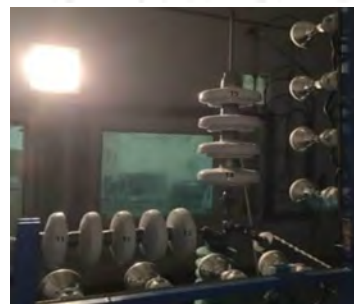
Figure 7: Test procedure and set up for the TERNA 2000h multistress ageing test
