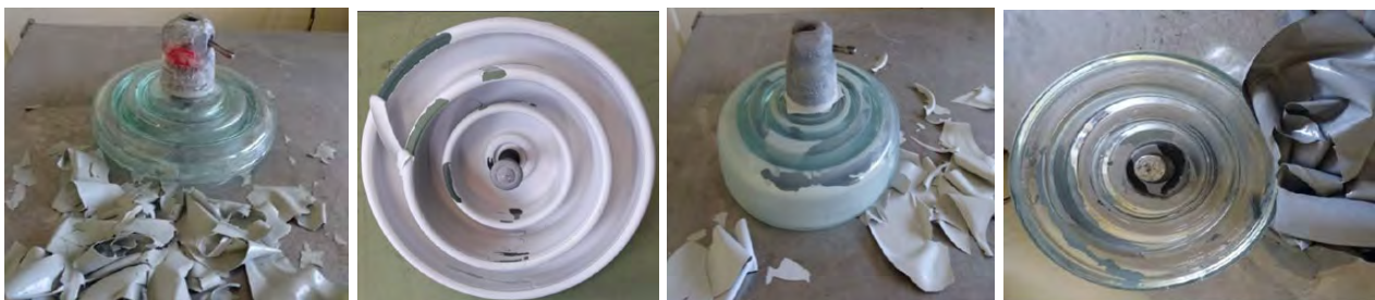
Figure 12: Various types of silicone coatings tested directly after being extracted from the boiling tank after 100h of immersion.
