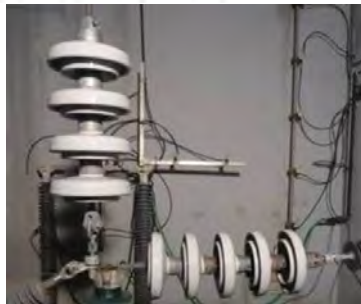
Figure 7: Test procedure and set up for the TERNA 2000h multistress ageing test
