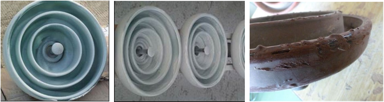
Figure 9: Examples of visual defects in the application. (left: uncoated areas, center: uneven coating, right: runners and droplets)
