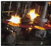
Automated pressing machine enables us to create complex glass shells.
