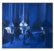
A toughening machine submits the glass shells to a rapid superficial cooling by blowing compressed air jets. The permanent compressive pre-stresses created on the surface of the glass shells increase considerably the mechanical resistance of the material.
