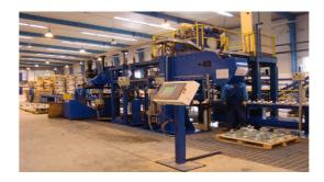
In 2008 a newly automatic control machine was developed in Sediver Shanghai to check each insulator by cameras and specific software before packing.
