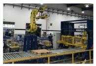
After QC acceptance, the insulators are packed, strapped onto pallets and stored.
