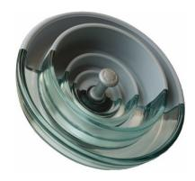
glass. This technology combines all the benefits of TGI with the hydrophobic properties of polymers. It is gaining acceptance by many US utilities dealing with contamination and has become a viable replacement for aging polymers. Depending on the pollution involved, a fully coated or undercoated shell has shown superb performance in severely polluted areas where washing was previously required.
