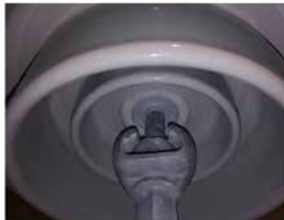
Middle & right: at the end of the test, the strong hydrophobicity and overall condition demonstrates the strong performance and lack of erosion on Sedicoat coated insulators after 2000 h multi-stress test
