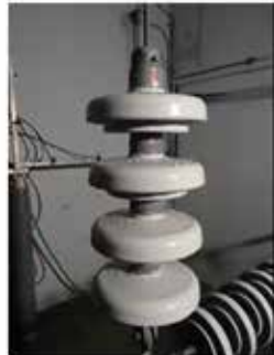
Middle & right: at the end of the test, the strong hydrophobicity and overall condition demonstrates the strong performance and lack of erosion on Sedicoat coated insulators after 2000 h multistress test
