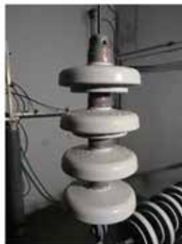
Middle & right: at the end of the test, the strong hydrophobicity and overall condition demonstrates the strong performance and lack of erosion on Sedicoat coated insulators after 2000 h multistress test
