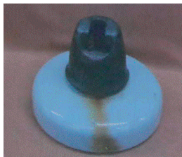
Rust appears on cap due to surface current
