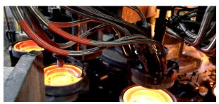
Automated pressing machine enables us to create complex glass shells.
