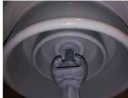
Middle and right: at the end of the test, the strong hydrophobicity and overall condition demonstrates the strong performance and lack of erosion on Sedicoat coated insulators after a 2,000-hour multi-stress test.
