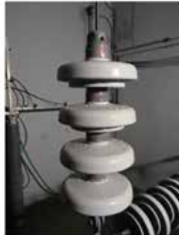
Middle and right: at the end of the test, the strong hydrophobicity and overall condition demonstrates the strong performance and lack of erosion on Sedicoat coated insulators after a 2,000-hour multi-stress test.
