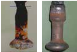
Corroded pin without zinc sleeve
