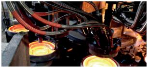
Automated pressing machine enables us to create complex glass shells.
