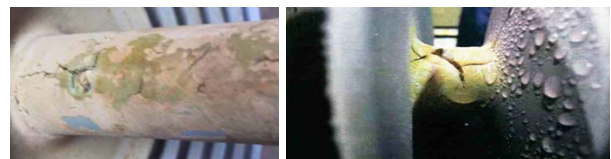
Figure 1: Left: erosion at shank near the fitting. Right: erosion between sheds.
