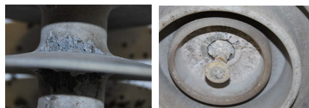
Figure12: condition of the insulators after 5 years in the test station (USCD= 66mm/kV) (*)
