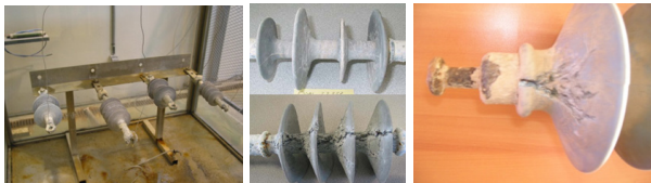
Figure 2: Left: clean fog erosion test chamber. Center: ATH filled silicone (top) and LSR (bottom) after 2000h in the chamber. Right: LSR eroded in coastal environment after less than 5 years in service (Morocco).
