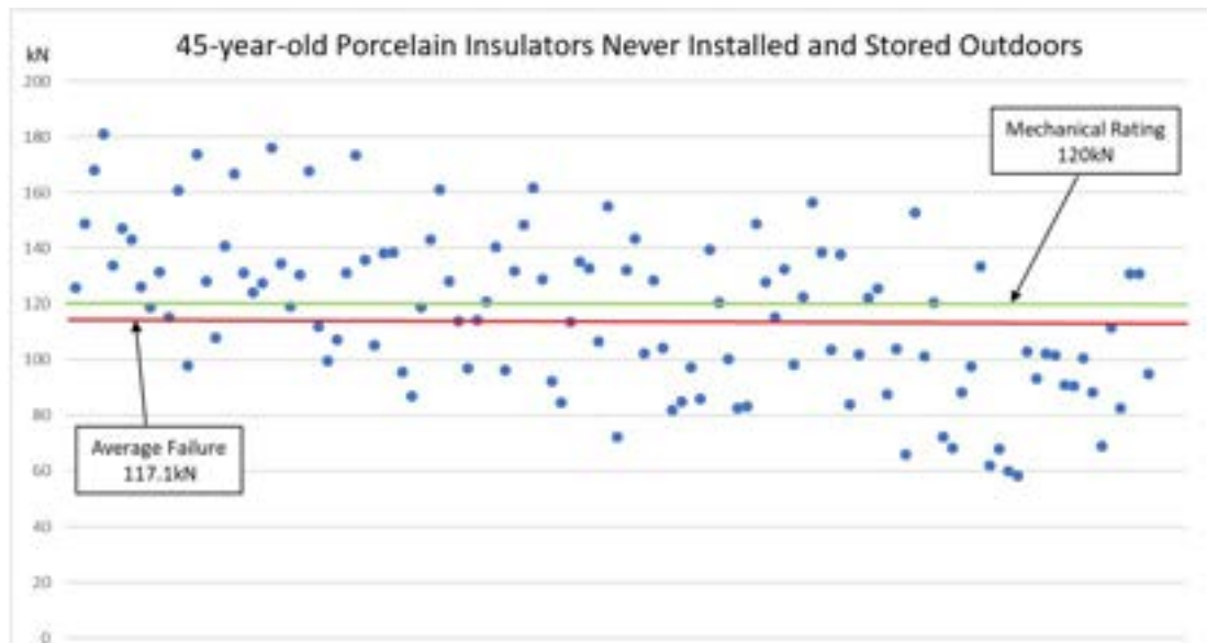
Figure 2 – M&E test results on unused porcelain insulators after 45 years in outdoor storage. The horizontal axis represents individual sample number, not timeline.
