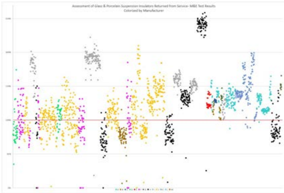
Figure 1B- Porcelain & toughened glass insulator M&E test results with unique colorization for each manufacturer included in the study. The horizontal axis represents individual sample number, not timeline.
