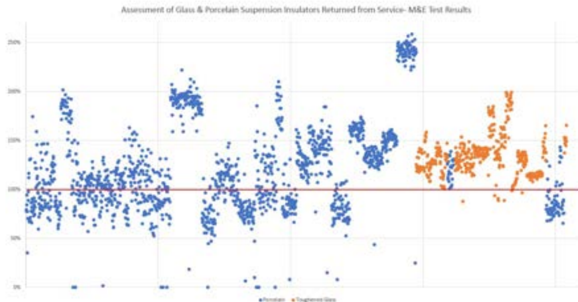
Figure 1A- Porcelain & toughened glass insulator M&E test results. Blue datapoints represent porcelain samples while toughened glass insulators are shown in orange. The horizontal axis represents individual sample number, not timeline.
