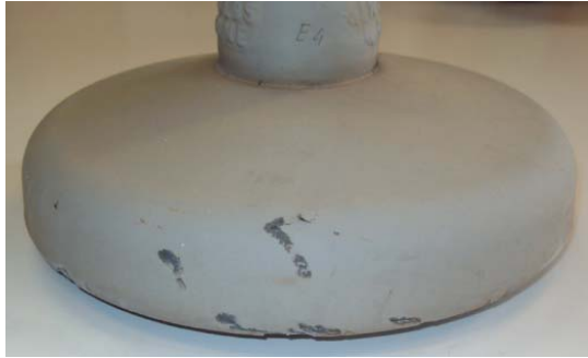
Figure 2. Example of RTV coating surface scrapes resulting from poor handling.
