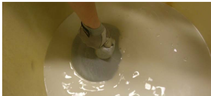
Figure 8. Example of contamination procedure by dipping of RTV-coated insulators: the insulator is manually rotated in the slurry to obtain uniform pollution layer
