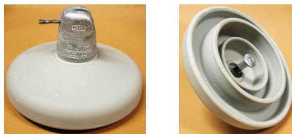
Figure 7. RTV-coated glass cap-and-pin insulator.
