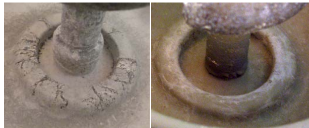
Figure 1. Example of the difference in behavior of two coating materials with different ATH and LMW contents when subjected to a salt-fog aging test.
