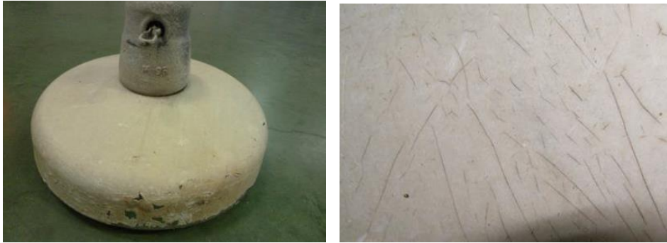
Figure 12: Silicone coated toughened glass insulator after 18 years in service
