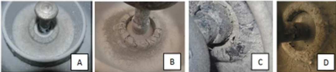
A: polymer 1 ATH type a B: polymer 2 ATH type b C: polymer 2 ATH type c D: polymer 2 quartz filler
