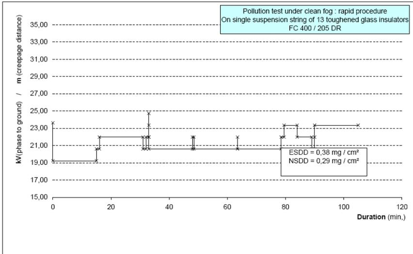
**Figure 3:** During the test time a slight washing effect of the solid layer pollutant after approximately 80 minutes under clean fog can be seen. The impact on the test value is less than 10%
