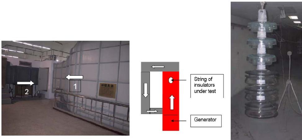
**Figure 10:** Dust wind tunnel test of “outerib” profiles
