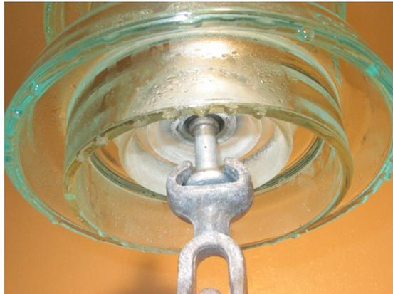
**Figure 8** : bottom view of the fog type after the salt fog test
