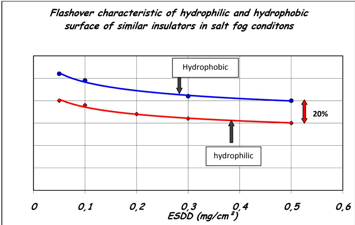
**Figure 13:** Salt fog test results on hydrophobic and hydrophilic surfaces
