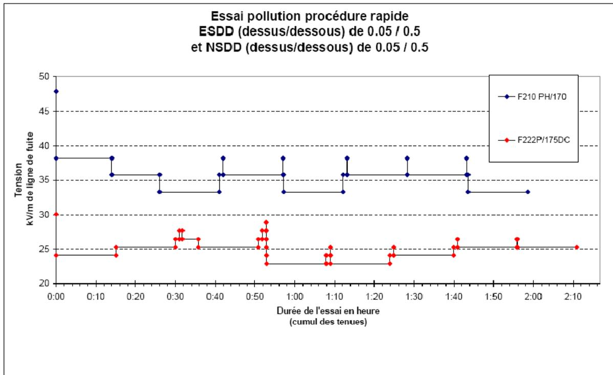
**Figure 12:** Test results from the clean fog type with two different types of insulators.
