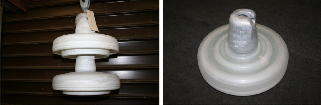
**Figure 4** : Solid layer deposit on toughened glass insulators using CEB application method.
