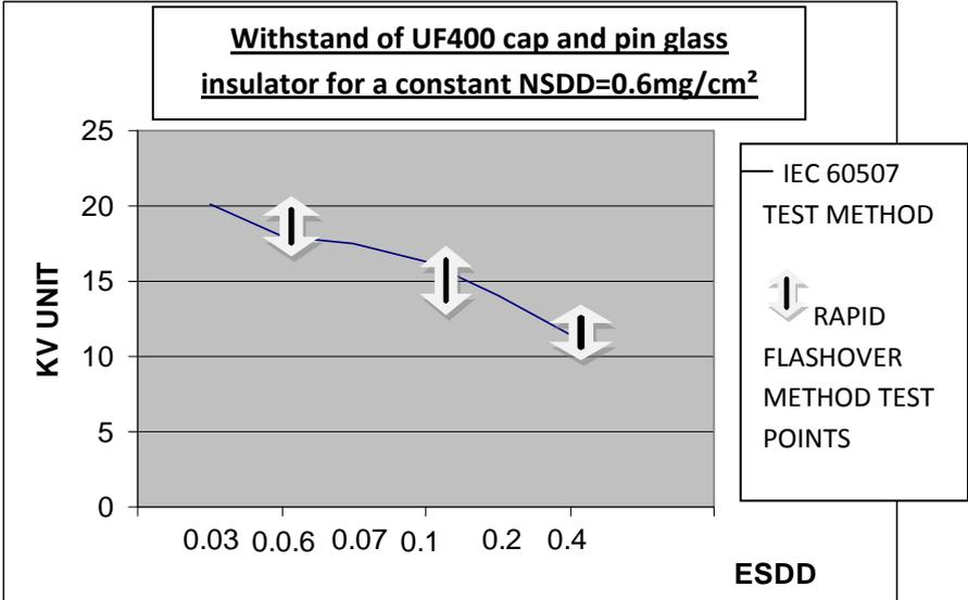
**Figure 5**: verification of the coherence between IEC 60507 method and rapid flashover method in the case of clean fog test protocol
