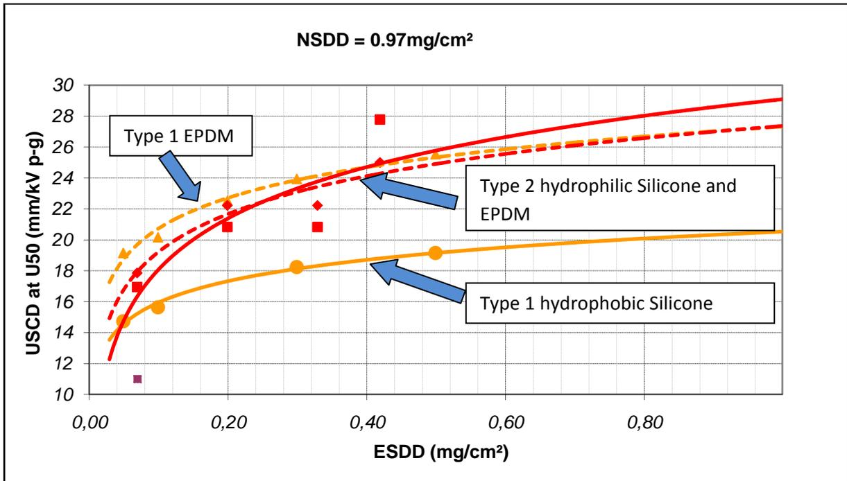
**Figure 14:** Solid layer contamination characteristic of various materials (USCD)
