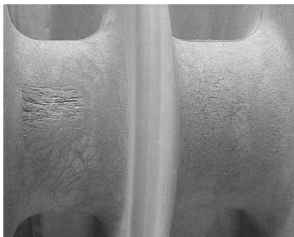
Figure 6 Erosion damage on L profile EPDM at 31 mm/kV.
