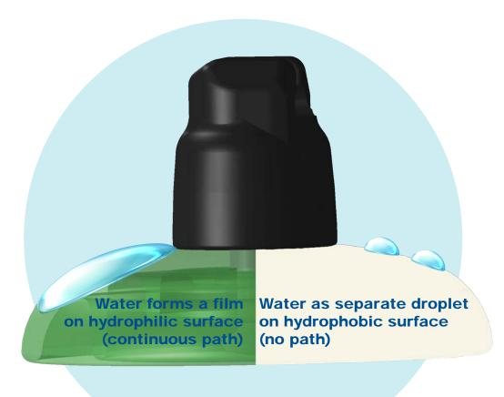
The hydrophobic water repellent property of the RTV coating keeps the water droplets apart on the surface of the insulator
