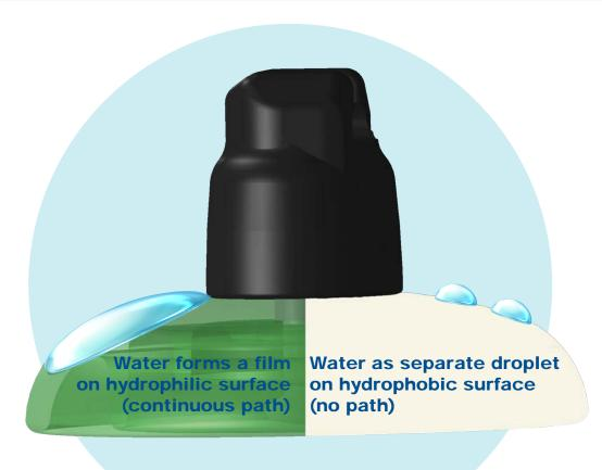
No formation of conductive water film on the surface of the insulator
