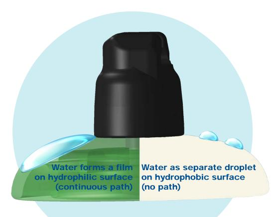
Leakage currents are reduced on the surface of the insulator
