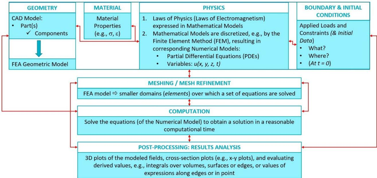
Fig. 1: Overall FEA Process Flowchart
