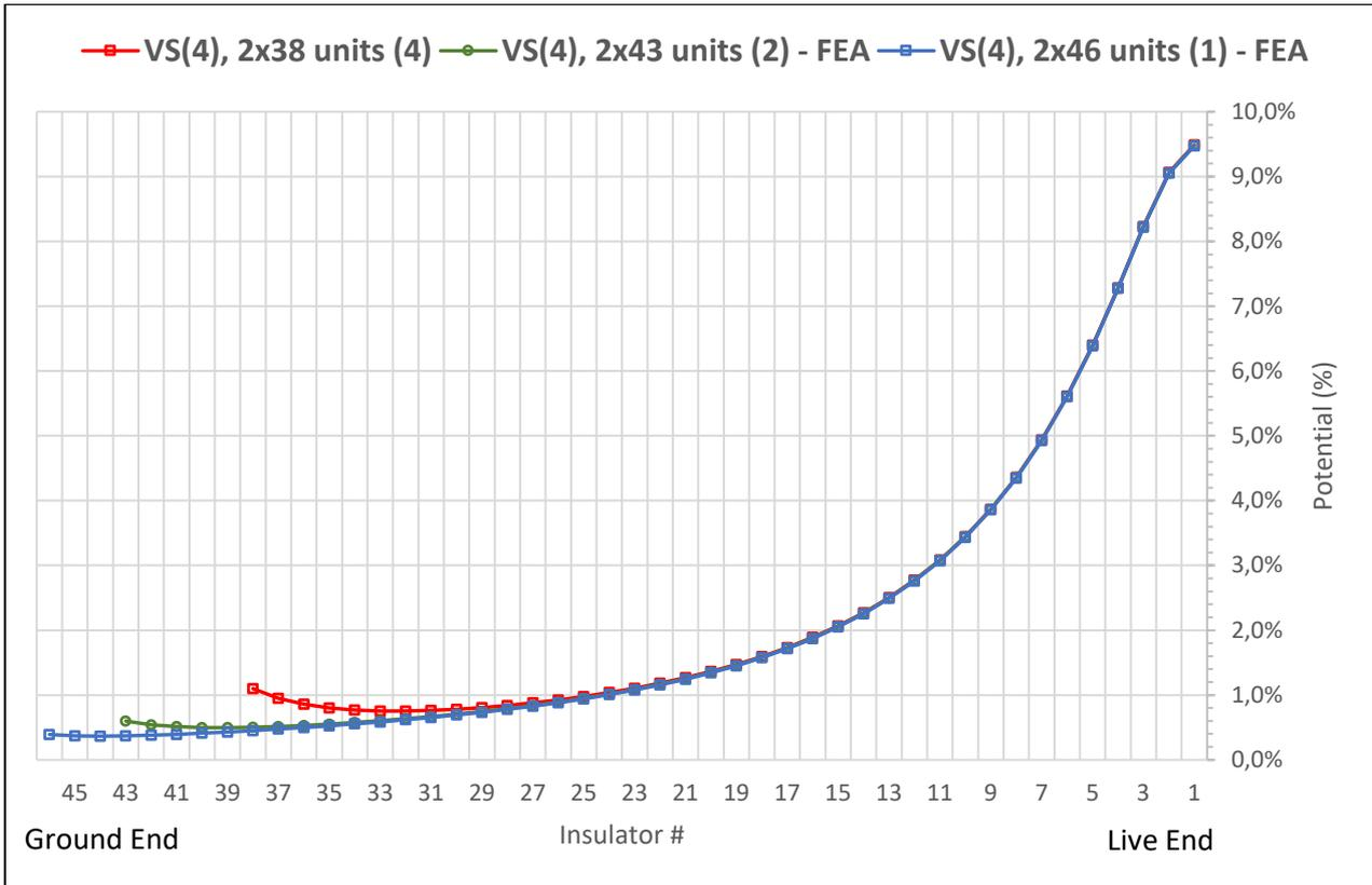
Fig. 13: FEA Computation of the voltage grading – Effect of the insulator unit number (N = 38, 43, or 46 units)
