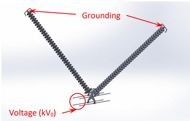
**Fig. 17A:** V-suspension set model without extension link and without tower.
