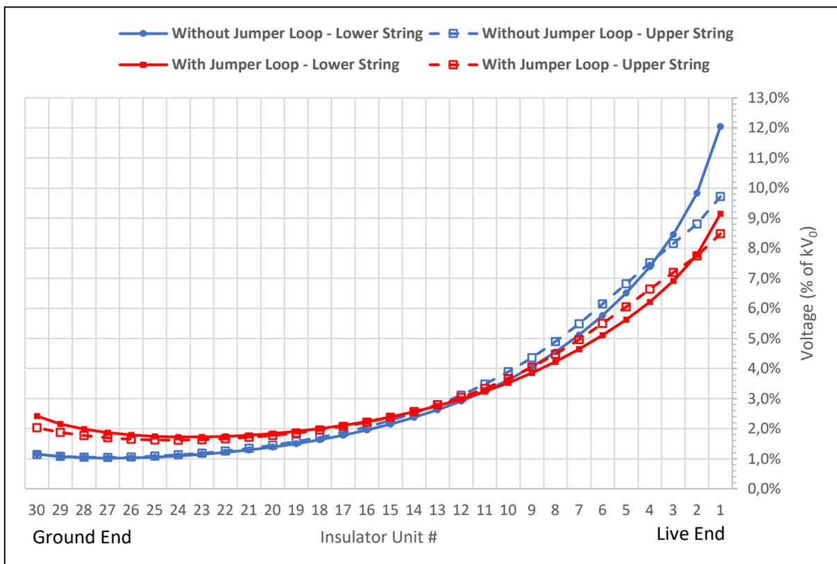
**Fig. 20:** FEA Computation of the voltage grading – Effect of the jumper conductor loop
