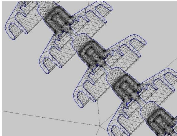
**Fig. 3:** “Standard” meshing of insulator units
