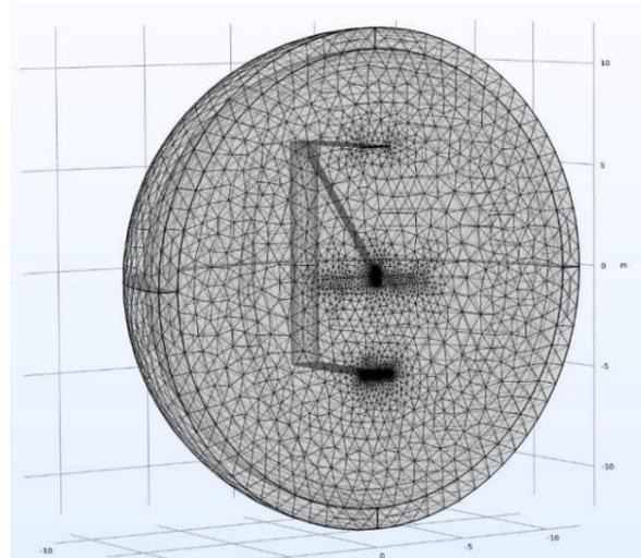
**Fig. 5B:** Meshing of the entire model
