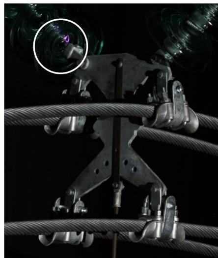
**Fig. 10B:** Corona Inception observed laboratory test (No protection)
