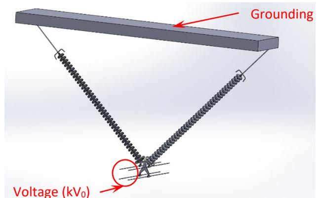
**Fig. 17B:** V-suspension set model with extension link and horizontal cross-arm.
