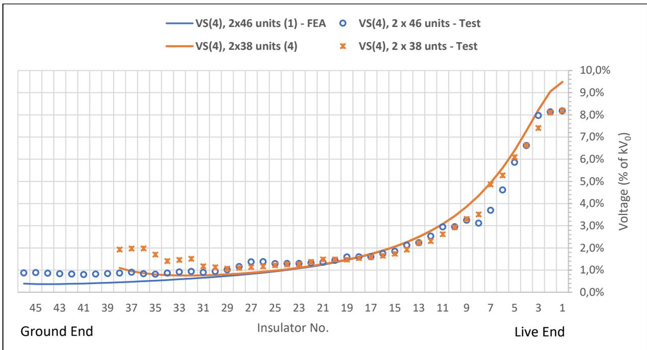
Fig. 14: FEA Computation vs. Measurement of the voltage grading – Effect of the insulator unit number
