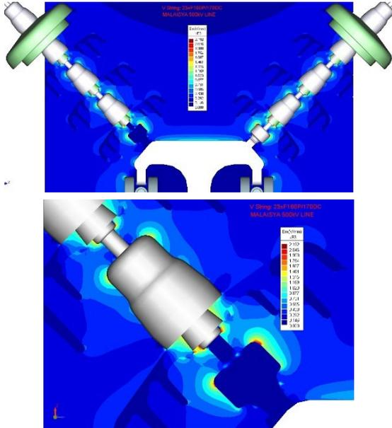
**Fig. 16A:** 2D-Plots of E-Field in the air at bottom insulators – Triple Bundle
