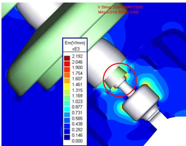
**Fig. 10A:** 2D-Plots of E-Field in the air on the first insulator unit (No protection)
