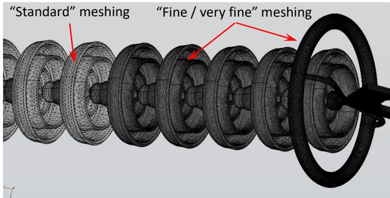
**Fig. 4:** Meshing adjustment at the bottom of the insulator string
