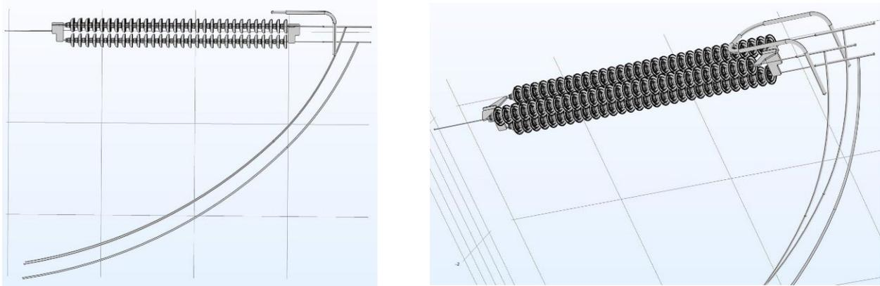
**Fig. 19:** Overall model of a triple tension set with jumper loop
