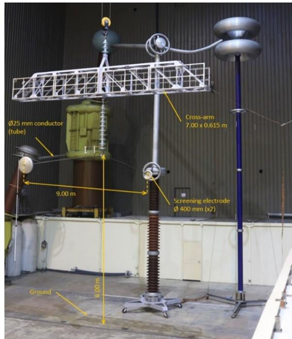
**Fig. 6B:** Overall view of the laboratory test set up (SEDIVER C.E.B. High-Voltage laboratory)
