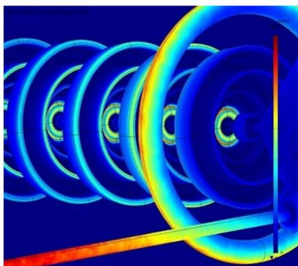
**E-Field distribution (kV/cm) on Surfaces at Live End (Top and Bottom views)**
