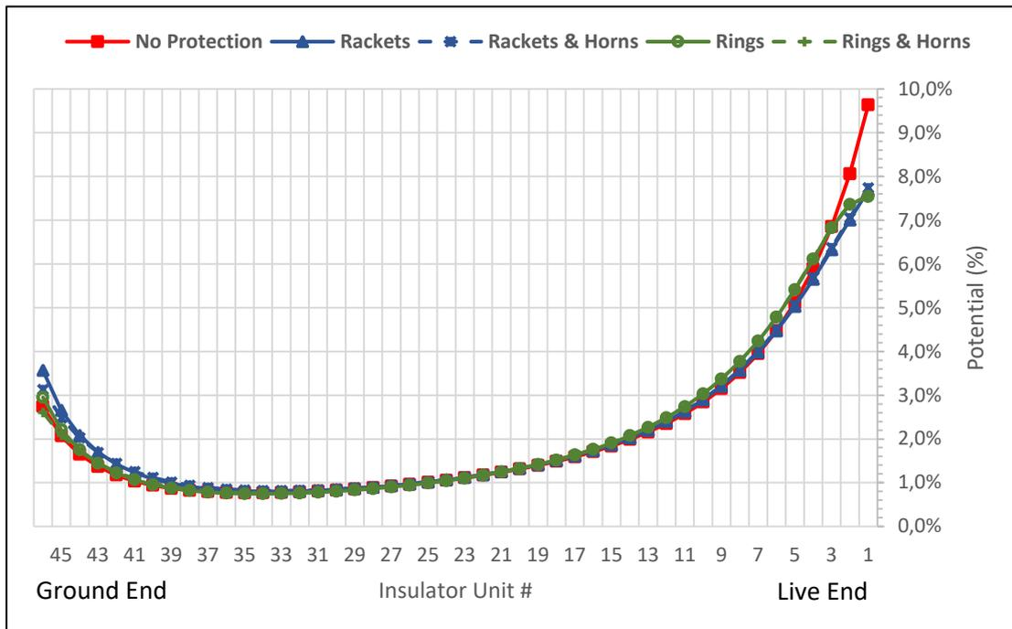
**Fig. 9:** FEA Computation of the voltage grading – Effect of the arcing protection devices
