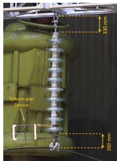
**Fig. 6E:** Single I-suspension set – Test
