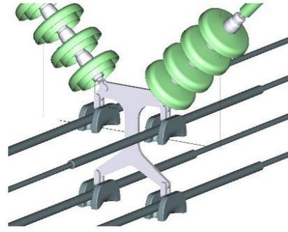
**Fig. 15B:** 3D Model with Quad Bundle.
