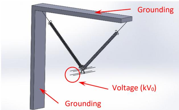
**Fig. 17C:** V-suspension set model with extension link, horizontal cross-arm, and vertical plane.
