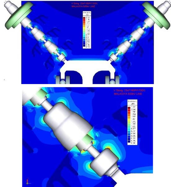
**Fig. 16B:** 2D-Plots of E-Field in the air at bottom insulators – Quad Bundle
