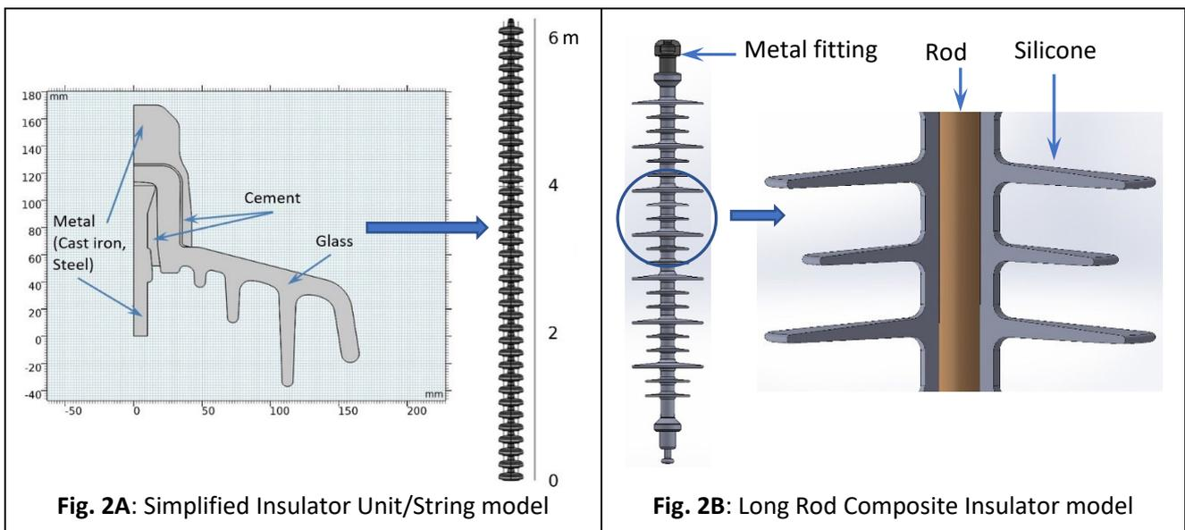
Some simplifications of this geometric model may become necessary but depend on the objective of the FEA. With regards to the assessment of Electric Field distribution and voltage grading along insulator strings,
