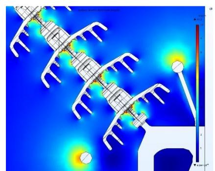
**Fig. 8:** Comparative views of the E-Field distribution (kV/cm) in the air around the insulator units at live end of the string (Cross-sectional views – Same scale)
