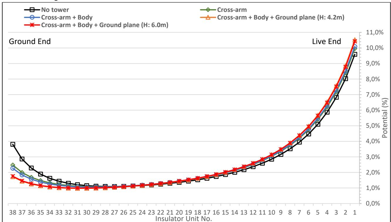
**Fig. 18:** FEA Computation of the voltage grading – Effect of the tower modeling
