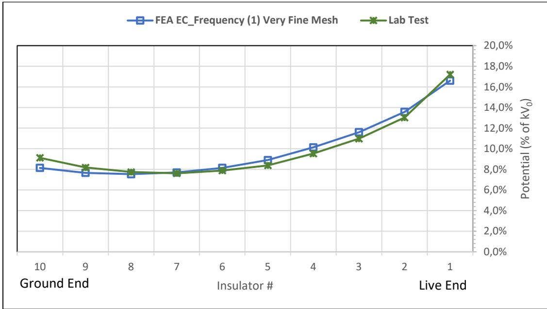
**Fig. 6F:** FEA Computation vs. Measurement of the voltage grading (% of the applied voltage)
