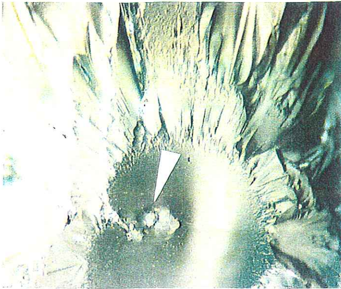
Fig. 5 - View of a detected inclusion
