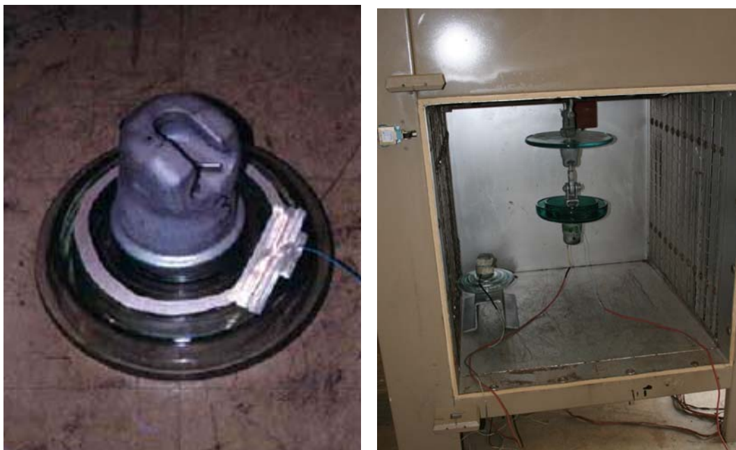
Figure 6: body resistance tests (CEB laboratory, France)
