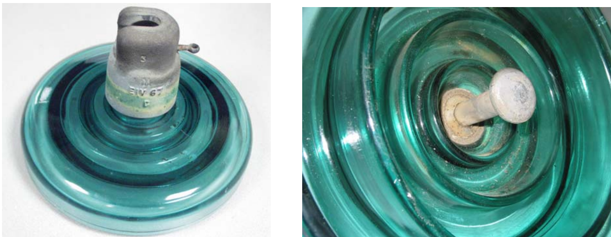
Figure 4: BPA 500kV DC insulators after more than 35 years in service. Mechanical rating is 180kN
