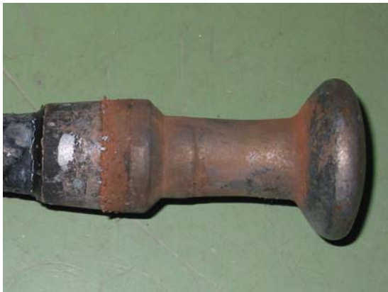
Figure 15 : condition of the pin removed after mechanical test. No corrosion
