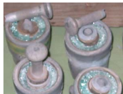
Figure 10 : residual strength test with preliminary thermal cycles (IEC 60797)
