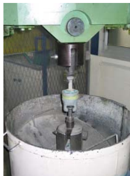
Figure 10 : residual strength test with preliminary thermal cycles (IEC 60797)
