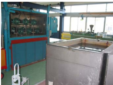
Figure 10 : residual strength test with preliminary thermal cycles (IEC 60797)
