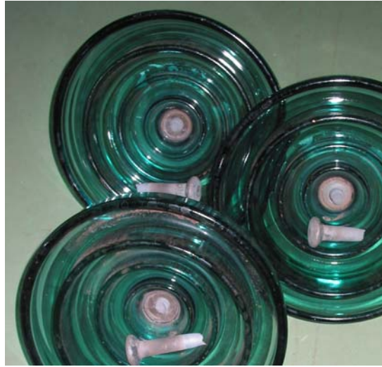
Figure 9 : Pin breakage typical of mechanical failure
