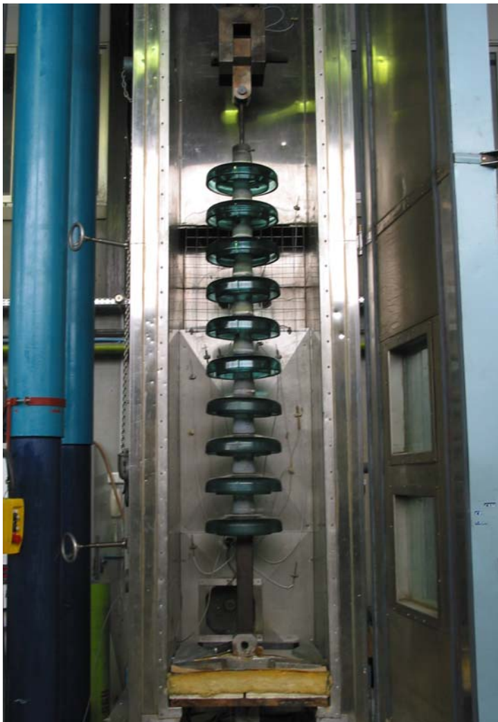
Figure 11: Thermo mechanical test -50/+50°C (Saint Yorre laboratory, France)
