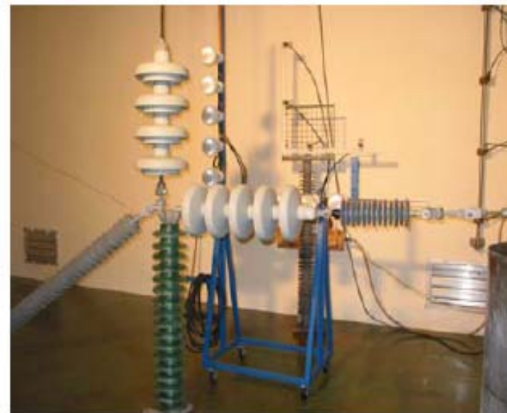
Controls and test chamber for Terna 2000h ageing test performed at Saint Yorre Laboratories
