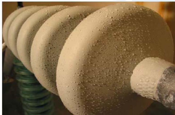
good hydrophobic behaviour after completion of the 2000h ageing test
