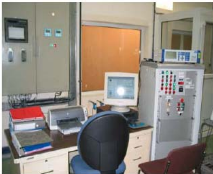
Controls and test chamber for Terna 2000h ageing test performed at Saint Yorre Laboratories
