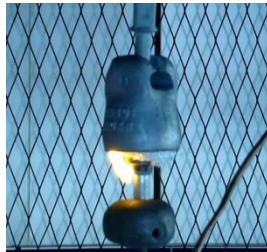
Figure 8: flashover of a stub
