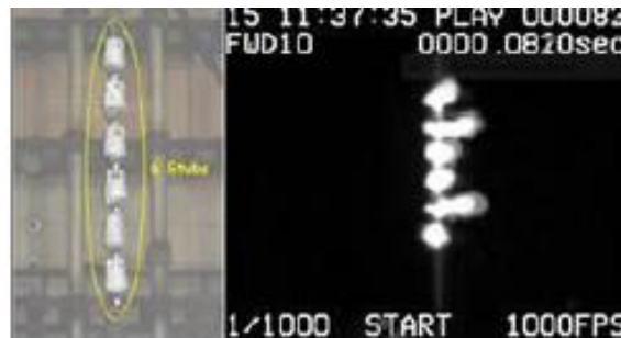
Figure 11: power arc on stubs
