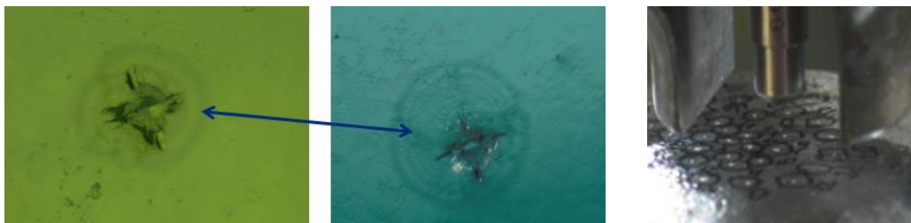
Figure 2: compressive strength measured on a new glass insulator (left) compared with the strength of a 50 year old unit (center) removed from service. Indentation measures (right) show a compressive stress in surface in the range of 200MPa to 210 MPa (approx. 30kpsi)
