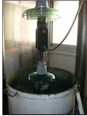
Fig11 - Insulator in traction machine
