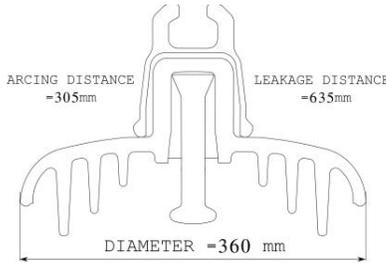
Fig. 4. Scheme of insulator UF300PU195
