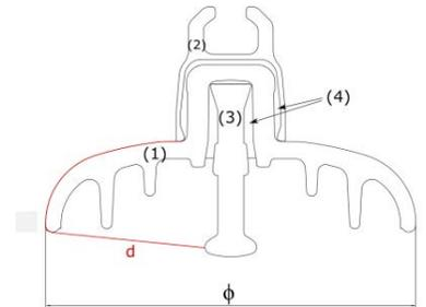
**Fig. 1.** Different parts of the insulator: (1) glass shell, (2) cap, (3) pin, (4) mortar. The outer diameter of the insulator is notated as  $\phi$  and the arcing distance as  $d$ .
