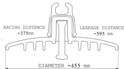
**Fig. 2.** Scheme of insulator UF300AN195
