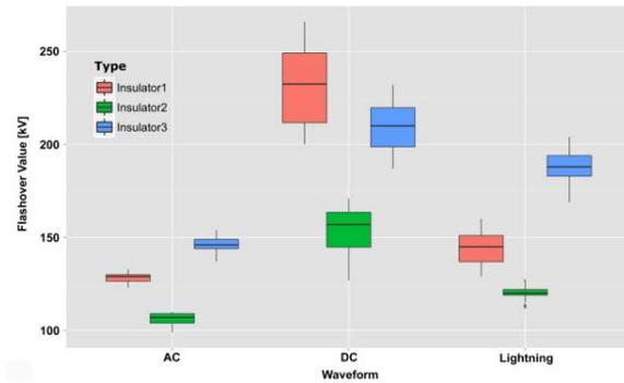
Fig. 8. Flashover voltage depending of the excitation mode. Positive and negative polarities are joined for DC and lightning.
