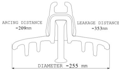
Fig. 3. Scheme of insulator UF120CB146
