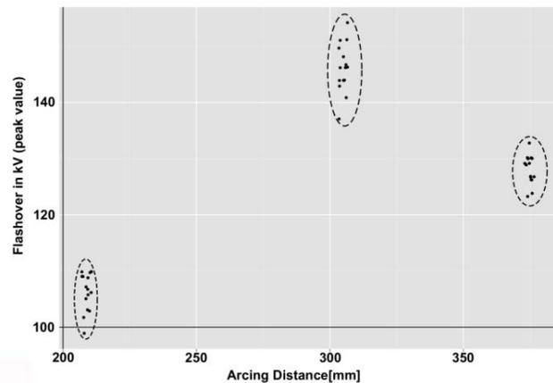
Fig. 6. Plot of the flashover voltage versus the arcing distance.
