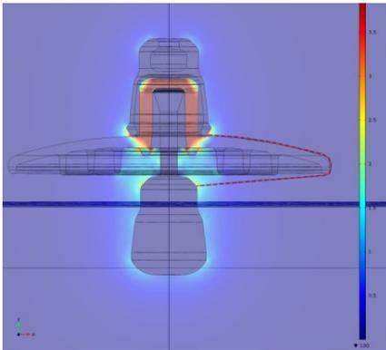
Fig. 5. The image shows the electric field solution in color grading and the path (red in dashed line) used for integrating. All other paths between the electrodes produce a higher flashover voltage.
