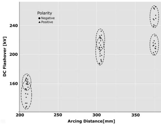
Fig. 7. Results for the DC case: vertical line is the flashover and the horizontal line is the arcing distance.
