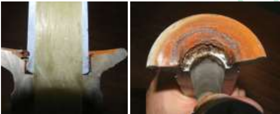
Figure 7: degradation at the triple point of a DC silicone composite insulator with corrosion of the fitting, disappearance of the seal and erosion of the rubber.
