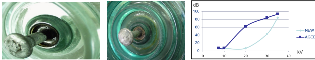
Figure 10: Unstable RIV performance based on non-permanent and artificial solution (left new insulator. Center: same insulator after 20h at 10g/l salt fog on a string of 6 units energized at 65kV. Right: RIV before and after the preconditioning).
