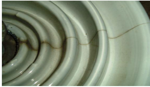
Figure 1: Example of radial crack in porcelain after Portland cement growth
