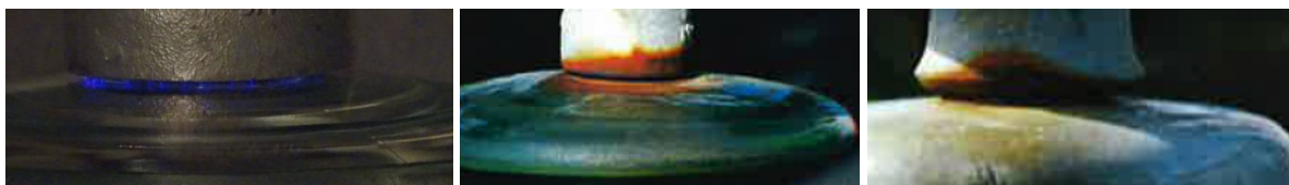
Figure 11: Large gap at the base of the cap leading to corona, corrosion of the cap base and high RIV
