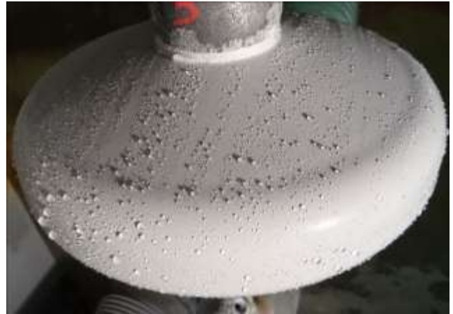
Figure 14: Insulator coated with newly developed SEDCO® coating at the end of the 2000 h multiple stresses ageing test according to TERN specification LIN-00J116 Rev. 1 dated 08/05/2013.
