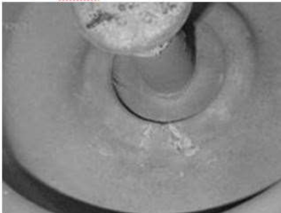
CE 2 : Signs of superficial erosion of the coating
