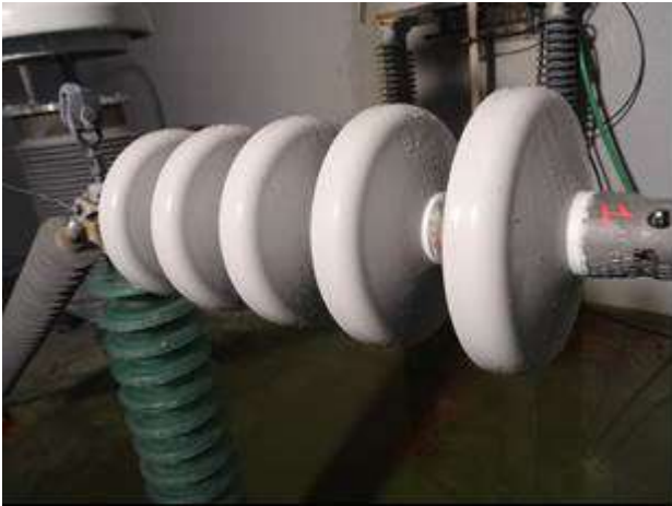
Figure 14: Insulator coated with newly developed SEDCO® coating at the end of the 2000 h multiple stresses ageing test according to TERN specification LIN-00J116 Rev. 1 dated 08/05/2013.
