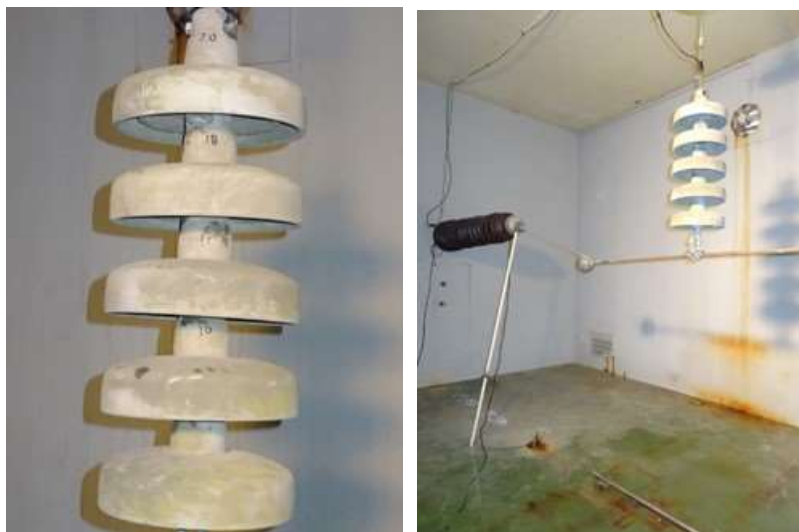
Figure 7: test set up for the clean fog test
