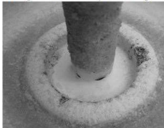
CE 3 : Localized erosion of the coating with spots where insulator surface is apparent
