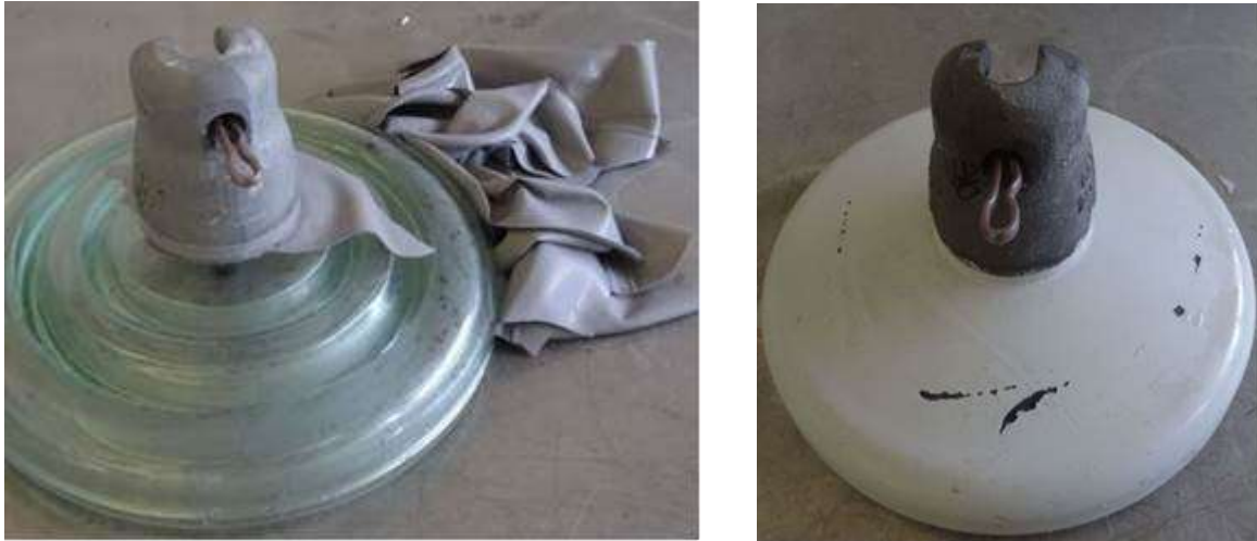
Figure 16: Results of 100 h boiling water test for a commercially available and for the newly developed Sedco® coating
