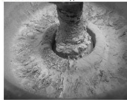
CE 5 : Delamination and erosion of the coating on large areas with large insulator surface visible
