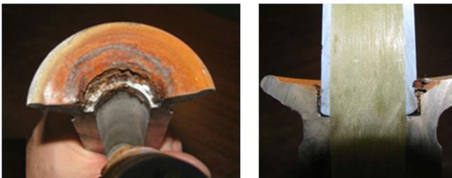
Figure 9. Corrosion and degradation of the seal of a polymer insulator at the triple point resulting in moisture ingress and major risk of failure. (removed from service after a decade)
