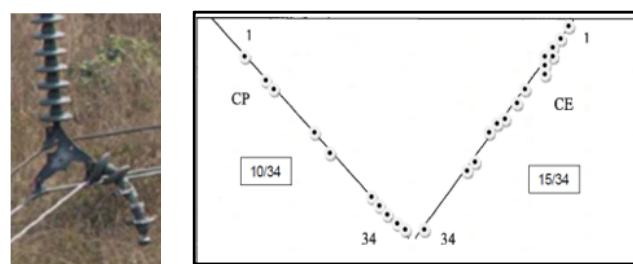
Figure 1. Left: String separation resulting from punctured porcelain. Right: Distribution of punctured discs in a porcelain Vee string in Congo on the 500kV DC Inga-Kolwesi line. Insulators did not have the body resistance required for a DC application. (30% failed units. Round circles show location of punctured discs found during the investigation).
