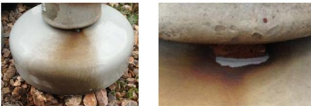
Figure 8. Damaged porcelain insulator resulting from the lack of zinc collar and excessive gap.
