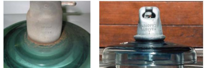
Figure 4. Left: Corrosion at the base of a cap without large zinc ring protection (Itaipu 1) - Right: Optimum design using a large zinc collar at the base of the cap
