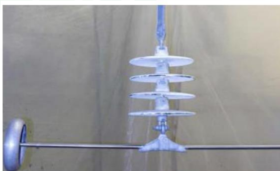
Non coated string : U50 = 73 kV 19 year old coated string: U50 = 240 kV (*)
