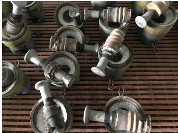
Figure 19: Overall aspect of the stubs after the mechanical test under heat conditions
