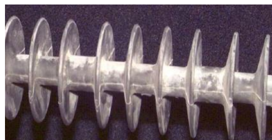
Figure 4: white powderish aspect of heated silicone
