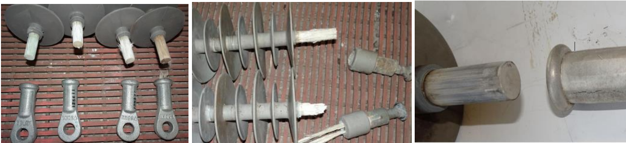
Figure 12: typical aspect of the tested units after the mechanical pull test
