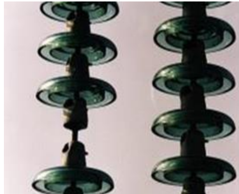
Figure 9 : typical aspect of a “stub”
