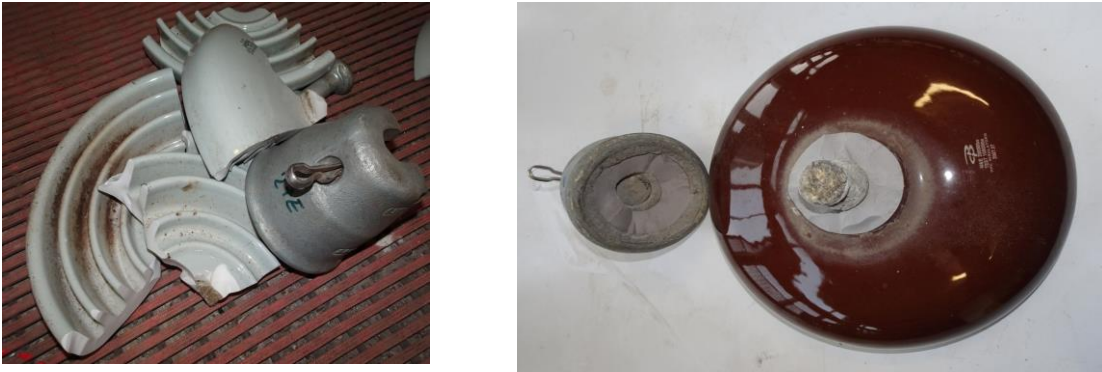
Figure 14: overall aspect of the insulators after the test
