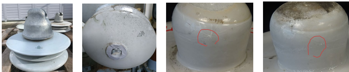
Figure 1. Porcelain outerib with dovetail head. Typical failures found in testing
