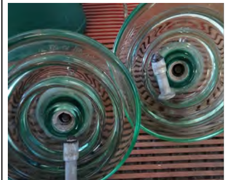
Figure 8 : Mechanical test results on toughened glass insulators and failure mode. (According to IEC and ANSI toughened glass insulators are only tested in mechanical mode and not M&E like porcelain since no internal puncture can take place)
