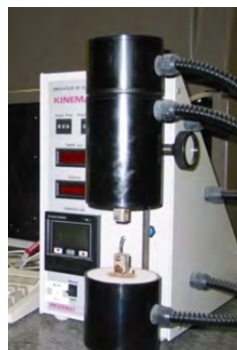
Figure 5 : drop of stiffness in a flexural test using a Trombotat (slice of rod placed between two clamps tested in torsion while the temperature is being increased).
