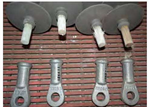
Figure 10 : Strong reduction of the mechanical strength of polymer insulators and typical failure modes
