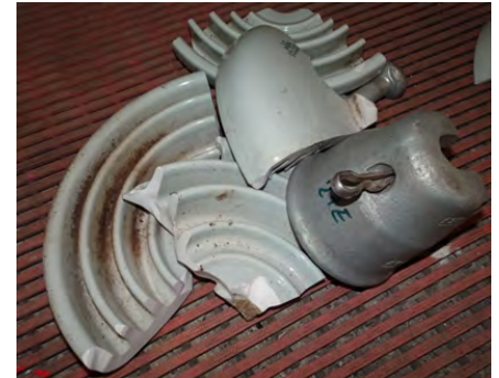
Figure 7 : M&E test results of porcelain insulators subjected to extreme temperatures for 3h
