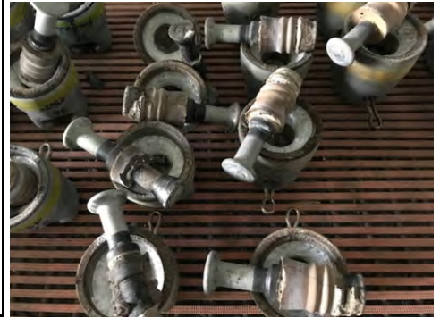
Figure 9: Residual strength test of toughened glass insulators under extreme heat and failure mode
