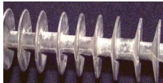
Figure 4: white powderish aspect of heated silicone
