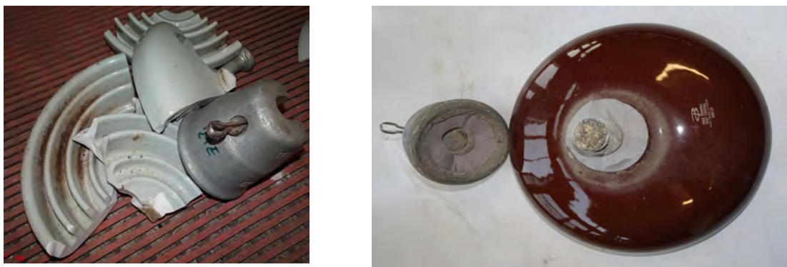
Figure 13: M&E test results of porcelain insulators subjected to heat prior to pull testing
