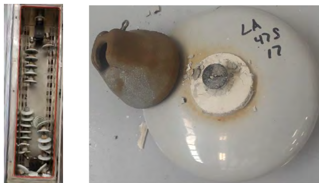
Figure 15: string separation during a thermo mechanical test performed on weak porcelain units containing already cracks from years of ageing.
