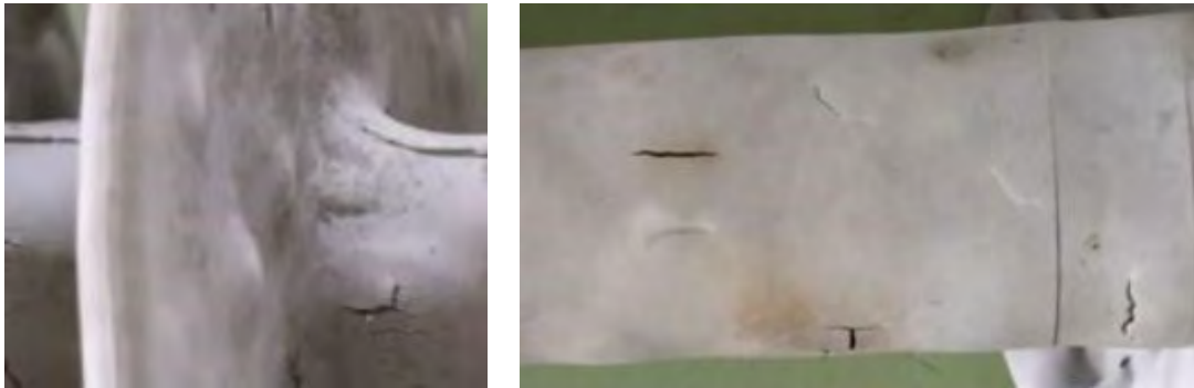
Figure21 : Cracks in silicone housing left after being subjected to heat for a few hours
