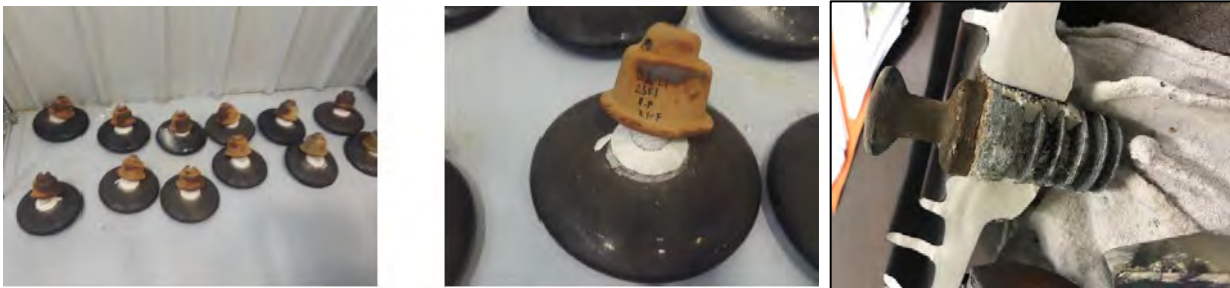
Figure 3: M&E test results on old porcelain from 1920 still passing the rated value; Average strength is at 13.4 kips with a standard deviation of 800 lbs. With 3 standard deviations the insulators are still good. The reason is mostly because of stable climatic conditions and an early 20th century over-designed product compared to the actual application.
