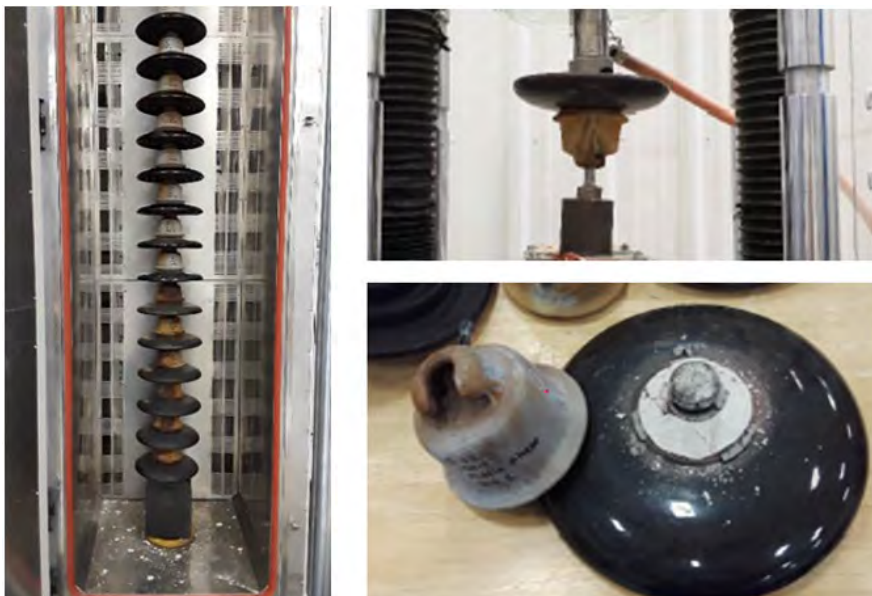
Figure 4: the M&E (right) of the same batch of insulators fails after a thermo mechanical test (left) as per ANSI 29 2B. Average failing load is at 10 kips (for a 11kips rating) with a standard deviation of 1500 lbs.
