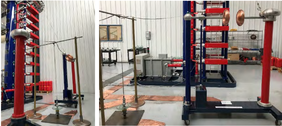
Figure 1: typical arrangement of steep front wave test with impulse generator and air gap. (Sediver West Memphis laboratory)
