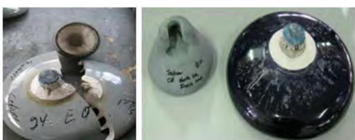
Figure and table 2: Mechanical results and standard deviations of 40 year old porcelain discs removed for testing from a 500KV line. The results do not show very low average values but huge variations and large standard deviations. The dispersion of the results was enough to consider that these units should be replaced rapidly.
